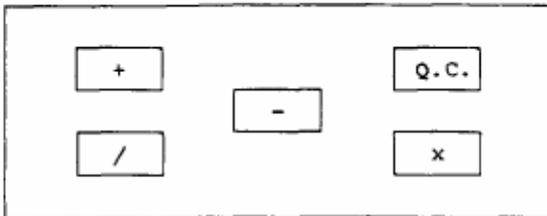
2. assembly lines in which all eight members are assigned to a specialized operation, and quality control is the last operation (Figure 3);
